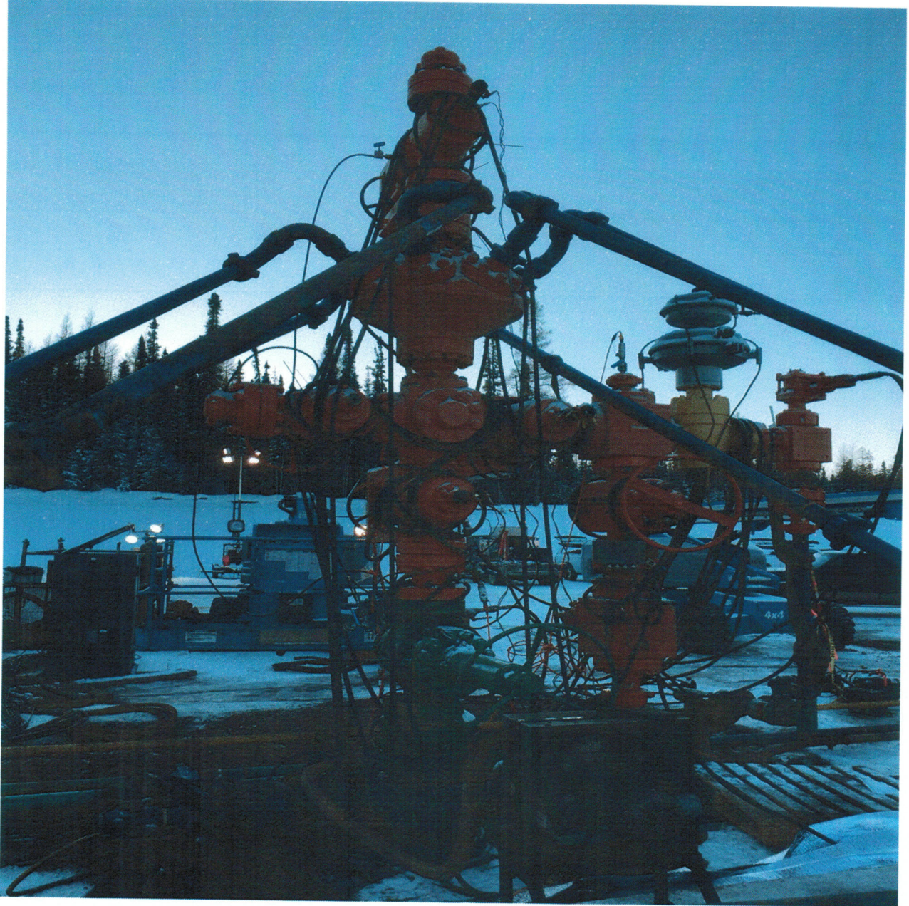
Example of job where once glycol lines were rigged in and wellhead tarped. This steam was rigged out.
